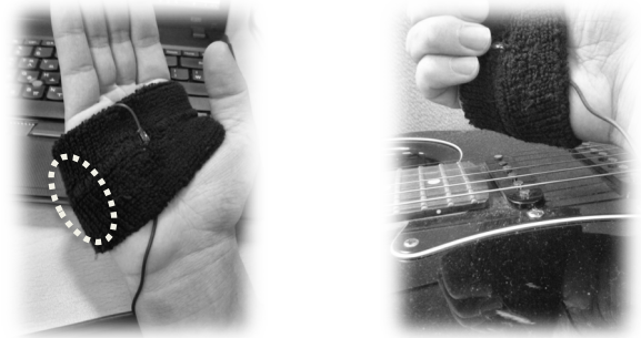
Figure 3 Installing an earphone to the player's hand. The coil of the earphone shown in the dotted circle generates the beacon signal to the guitar pickup of electric guitar (posing like a Karate Chop).
