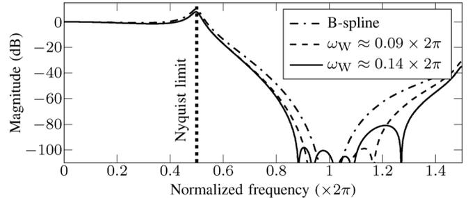
Fig. 1. Post-equalized (pole at  $-0.9$ ) amplitude response of the optimized four-segment third-order BLIT polynomial-spline when the design bandwidth  $\omega_W$  is  $80\pi/441 \approx 0.09 \times 2\pi$  (dashed line) and  $120\pi/441 \approx 0.14 \times 2\pi$  (solid line) for the baseband and the first two generations of aliasing. The response of the third-order B-spline polynomial (dash-dotted) is plotted for reference.
