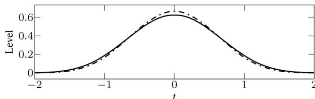
Fig. 2. Polynomial basis functions in the time-domain: B-spline (dash-dotted line) and the optimized polynomial-spline  $g(t)$  obtained with  $\omega_W = 120\pi/441$  (solid line).
